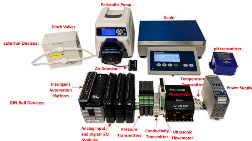
Annotated picture of an example setup of devices connected to an IAP
